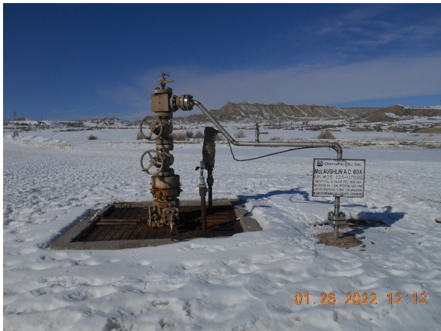
Injection wellhead
