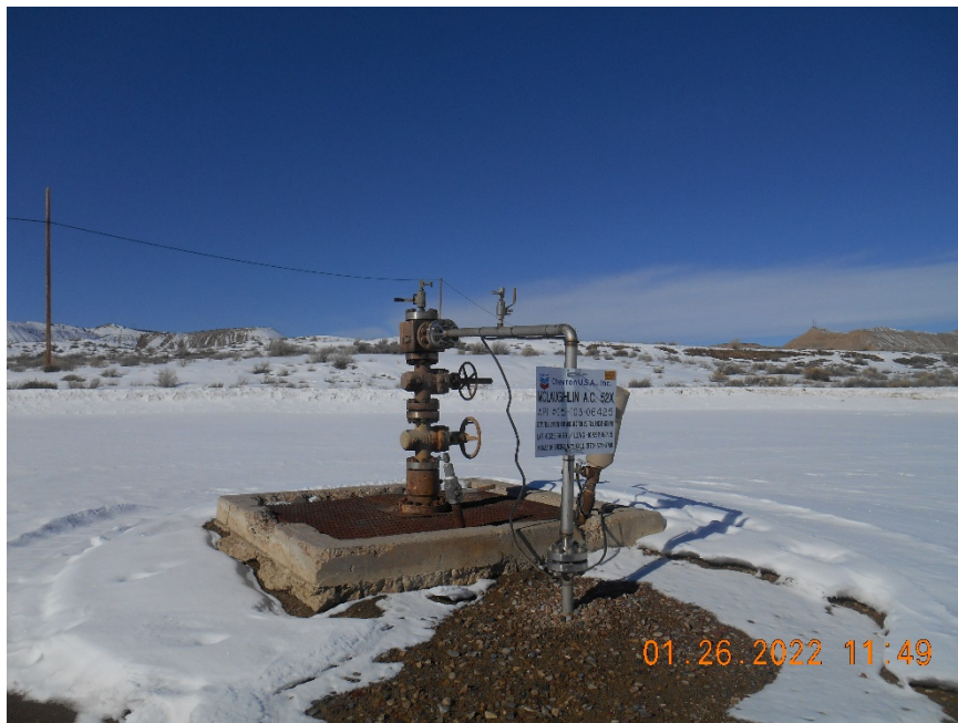
Injection wellhead
