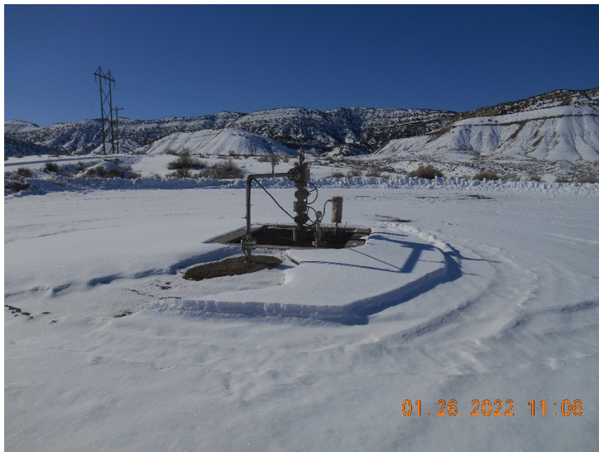
Injection wellhead
