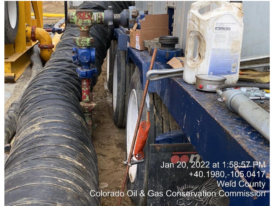
Photo #6 Not Adequate grounding on north Frack tanks/ Equipment
