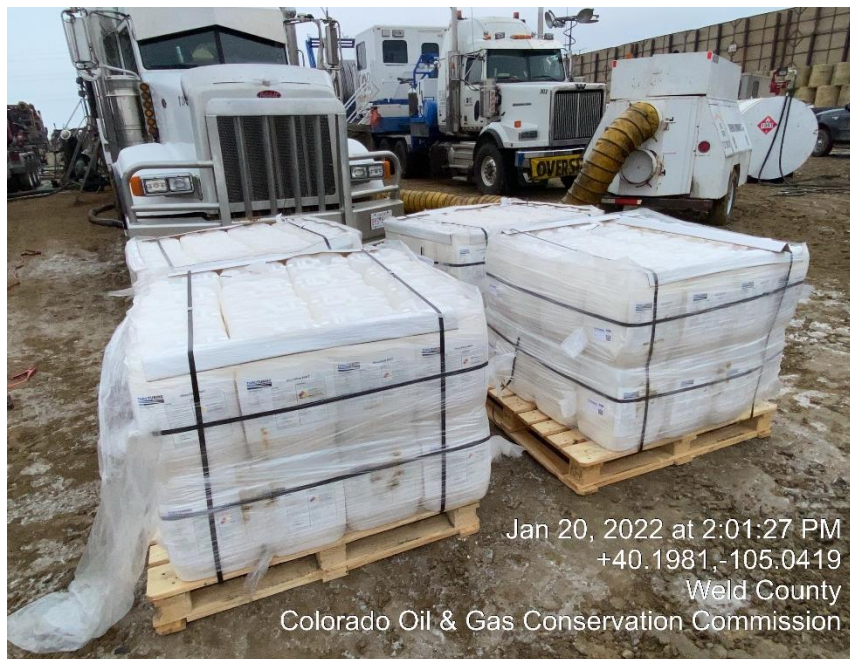
Photo #9 Not on secondary containment
