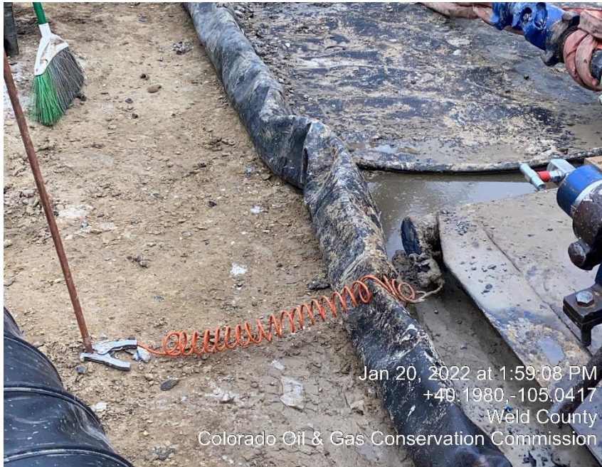
Photo #5 Not Adequate grounding on north Frack tanks/ Equipment
