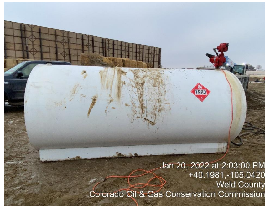
Photo #10 Not on secondary containment
