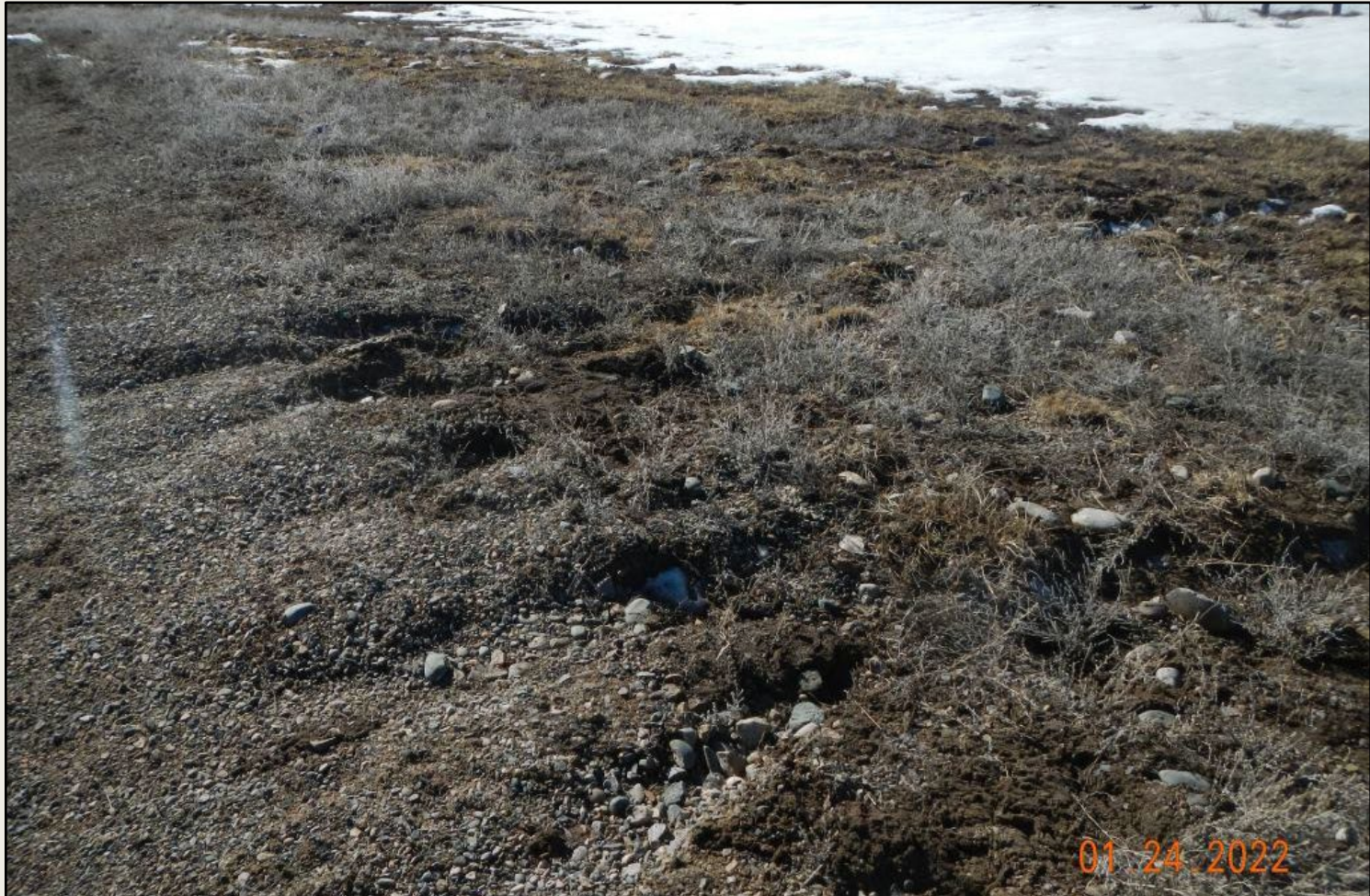
Photo 4. View of erosional rilling observed along the western edge of the working area and in the fill slope.
