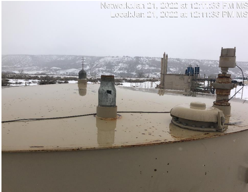
Photo #5757 Vent pipe on tank open ended.
