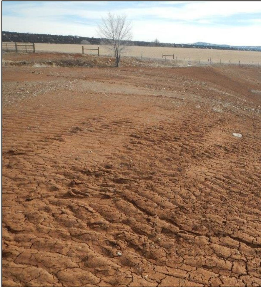
Photo 5. View of bare soils and erosional channeling (inset), up to 10 inches wide and deep within the southern project area. Bare and eroding soils need stabilization here.
