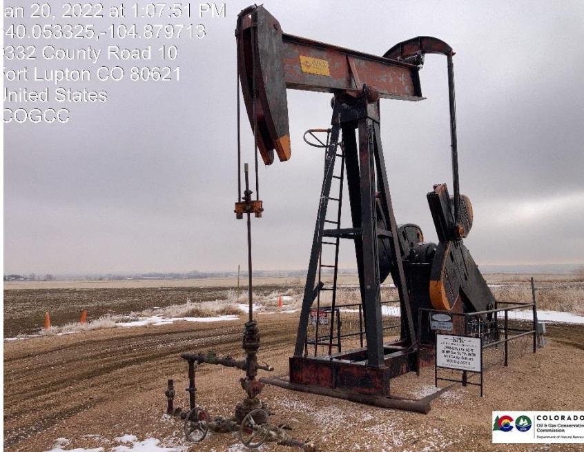
Pic 1 Wellhead , pumping unit
