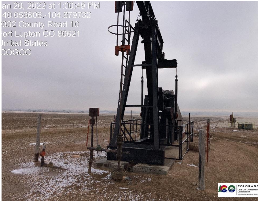
Pic 1 Wellhead, pump jack, electric equipment.
