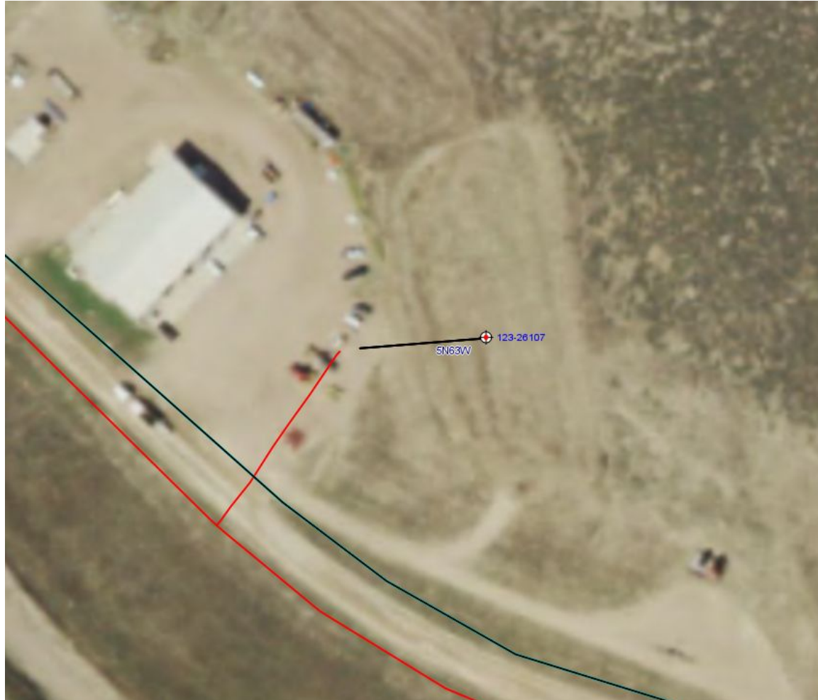
Photo 3. COGCC GISOnline aerial imagery with the flowline layer on illustrates that the remaining unused equipment (gas meter run and riser) is related to the PA well.
