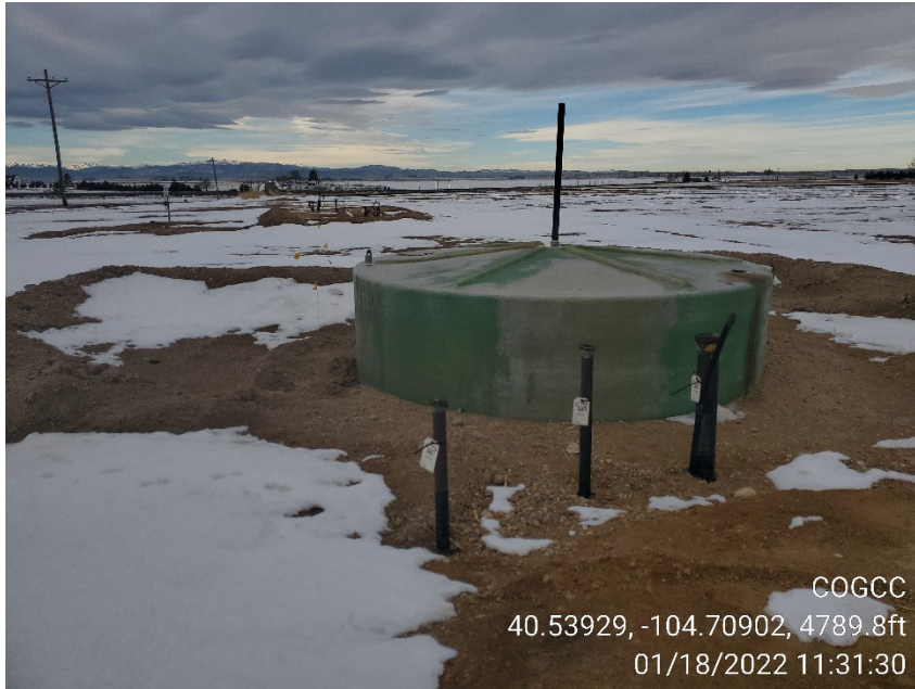
Photo 3 Partially buried vessel and unused flowline risers
