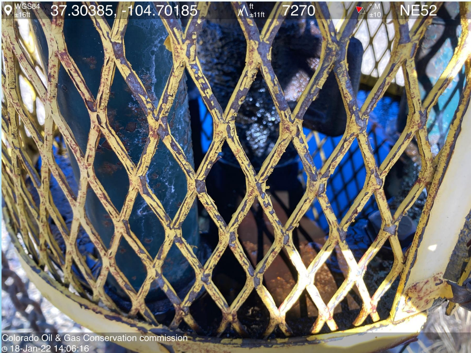
PHOTO 5: THERE IS WHAT APPEARS TO BE OIL POOLING ON BOTTOM PLATE OF DRIVEHEAD.
