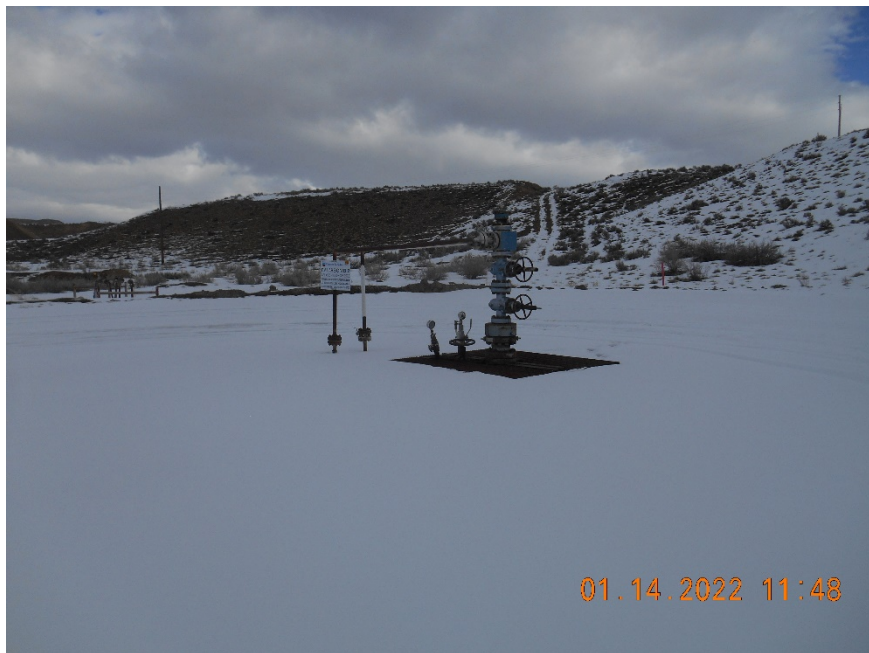
Injection wellhead-Temporarily abandoned.
