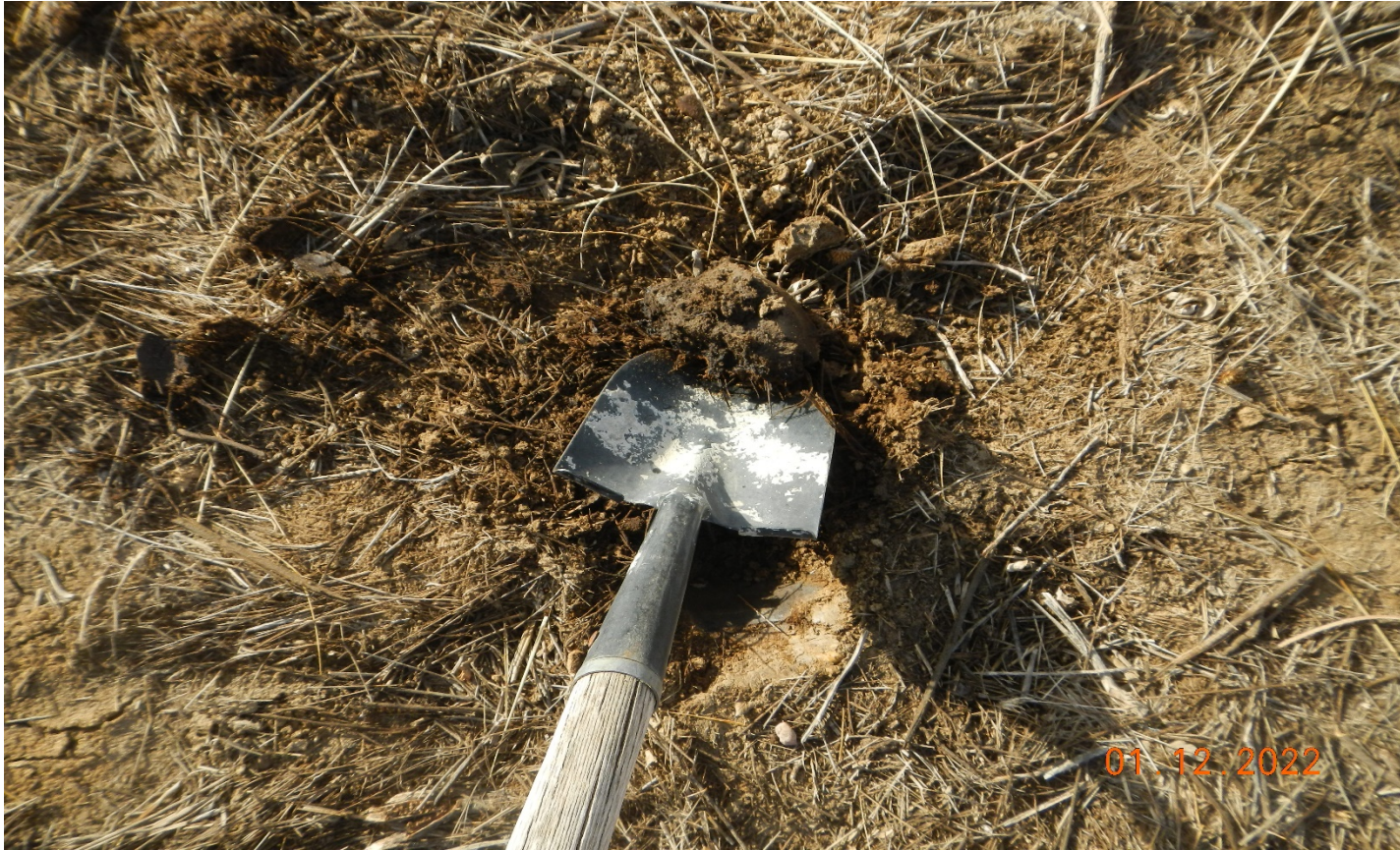
Photo 6. The soil at the spill area was dug a few inches down to show oily soils. The contaminated soils have not been cleaned up and removed.
