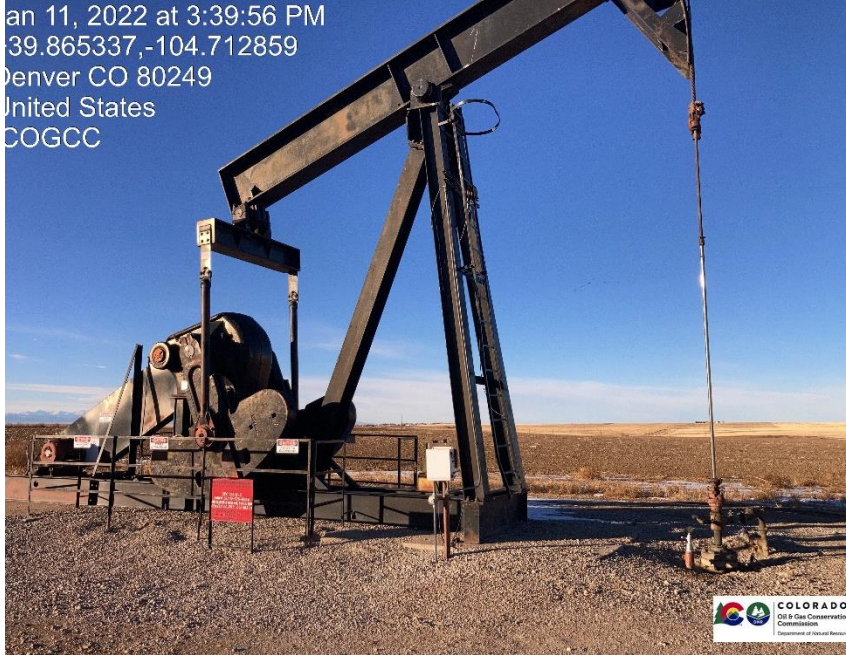
Pic 1 Wellhead / pumpjack
