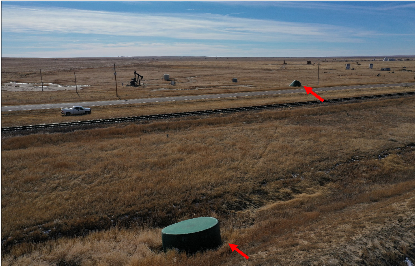
Photo 3. The top of the fiberglass tank blew across the highway.
