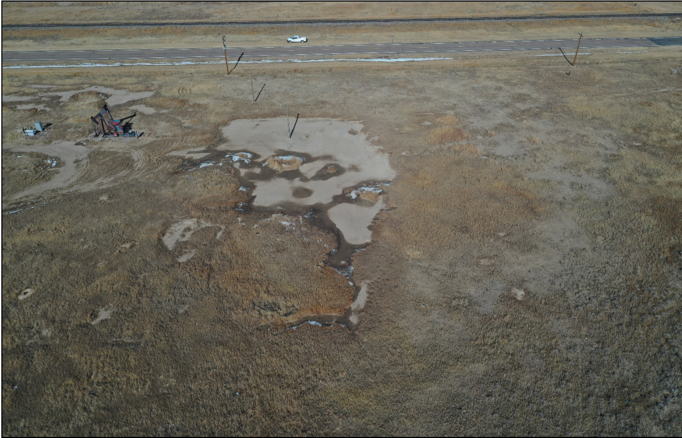
Photo 1. Drone aerial photo facing down toward the plugged and abandoned well site. The area around the abandoned site is bare of vegetation which indicates impacted soils from oil and gas operations.
