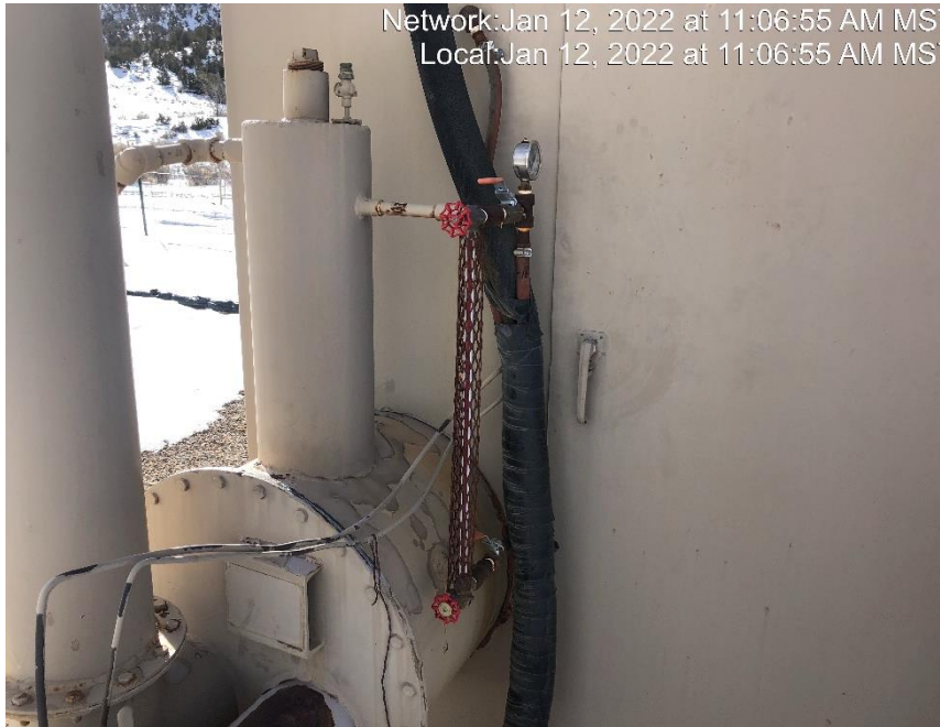
Photo #5655 Sight glass indicates the storage tank is full of an unknown fluid.
