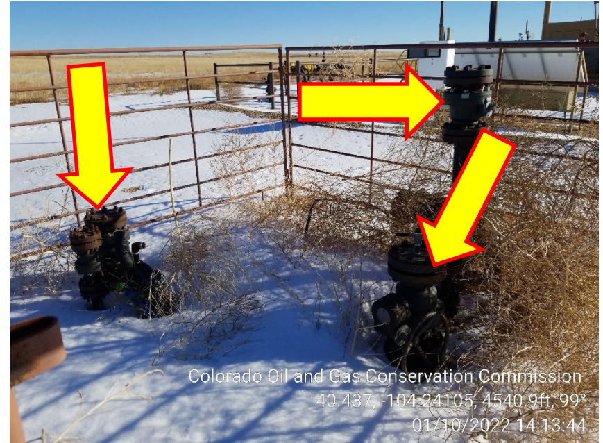
Photo 14 – Unmarked Risers
