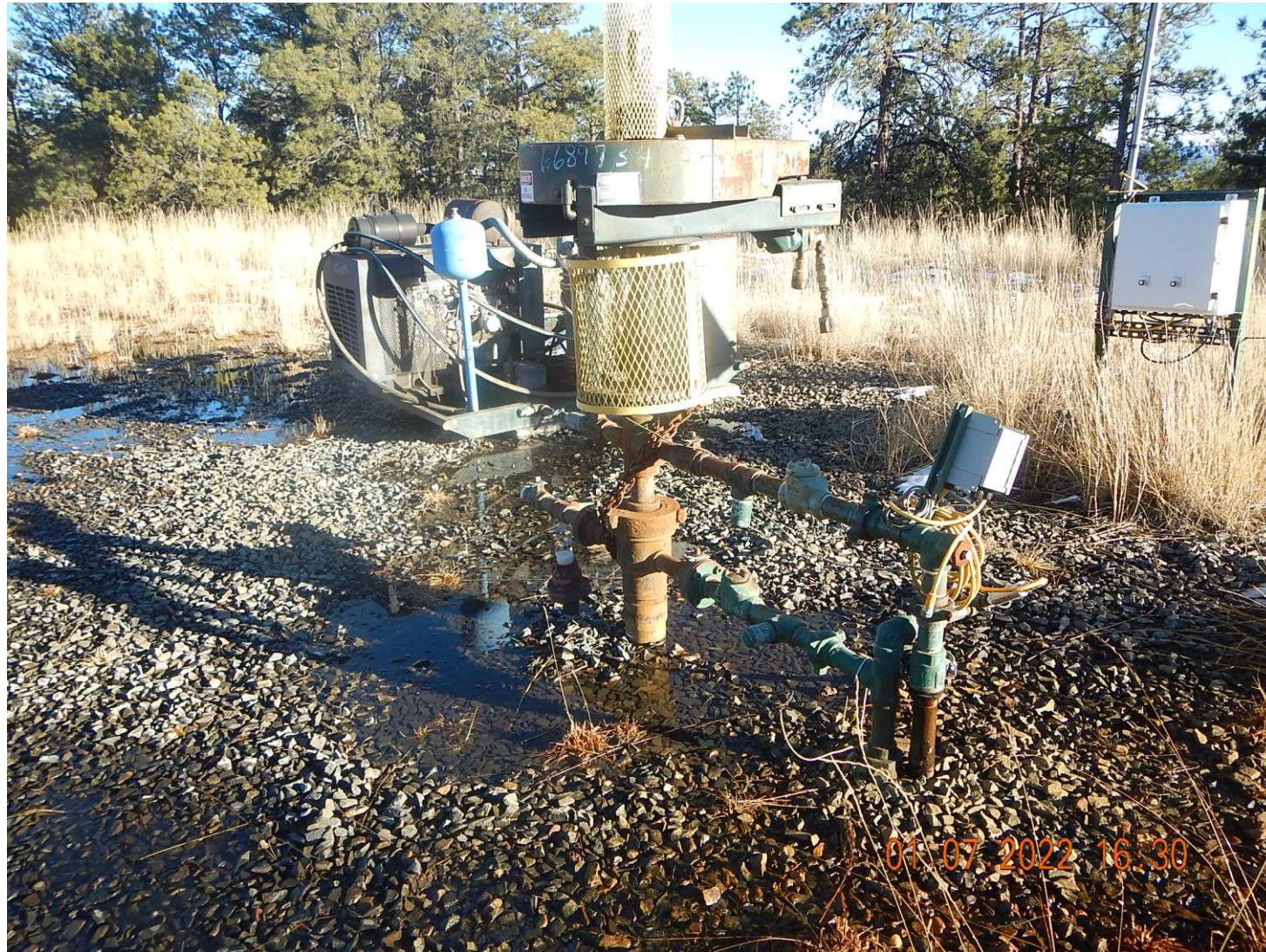
1. Spill source at the wellhead
