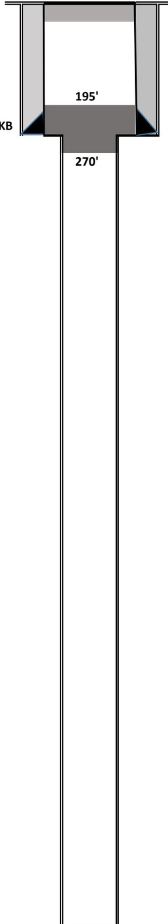
Cut off Csg 4' Below Mine Floor
