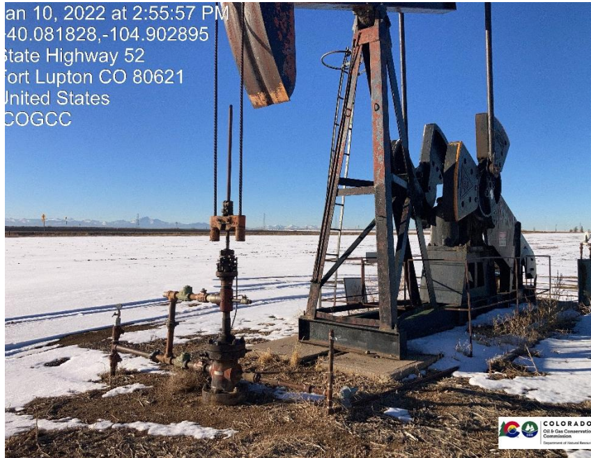
Pic 1 wellhead / pump jack
