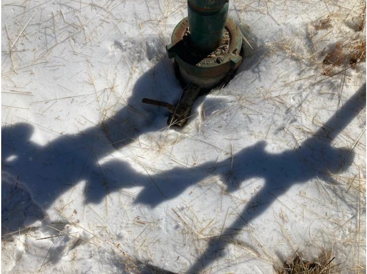
Installed appropriate fittings to allow bradenhead visual inspection as per Rule 419.a.(1),(2).
