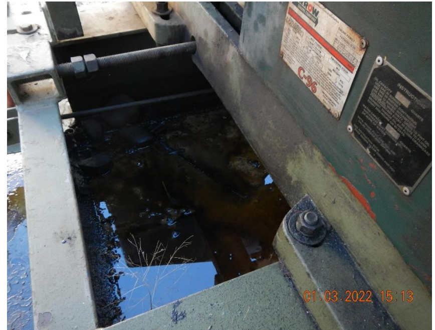
Fluid present beneath prime mover.
