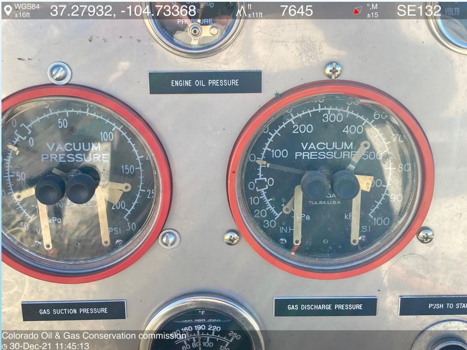
PHOTO 3: WELL IS BEING OPERATED ON A PARTIAL VACUUM.
