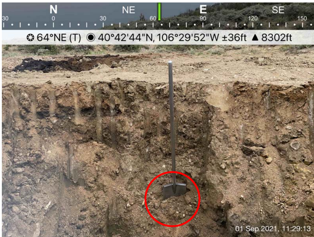
Photo 4: SS04, collected from base of flowline excavation, Margaret Spaulding (OWP) #12-A, 9/1/2021.
