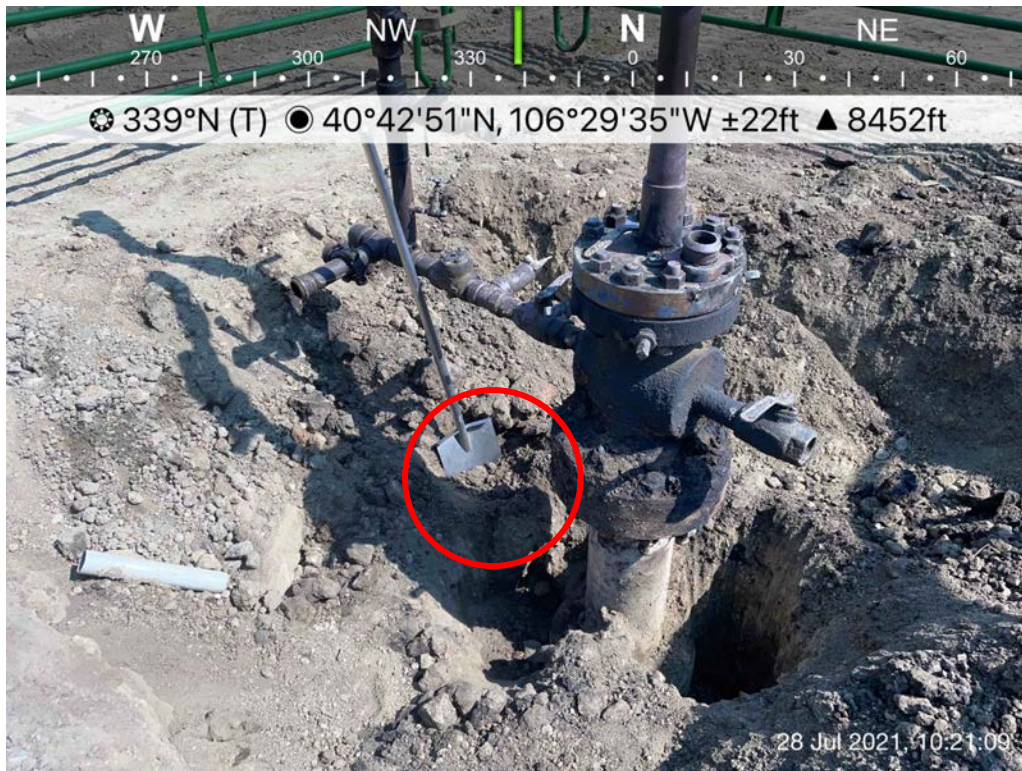
Photo 1: SS01, collected adjacent to Margaret Spaulding (OWP) #7 wellhead, 7/28/2021.
