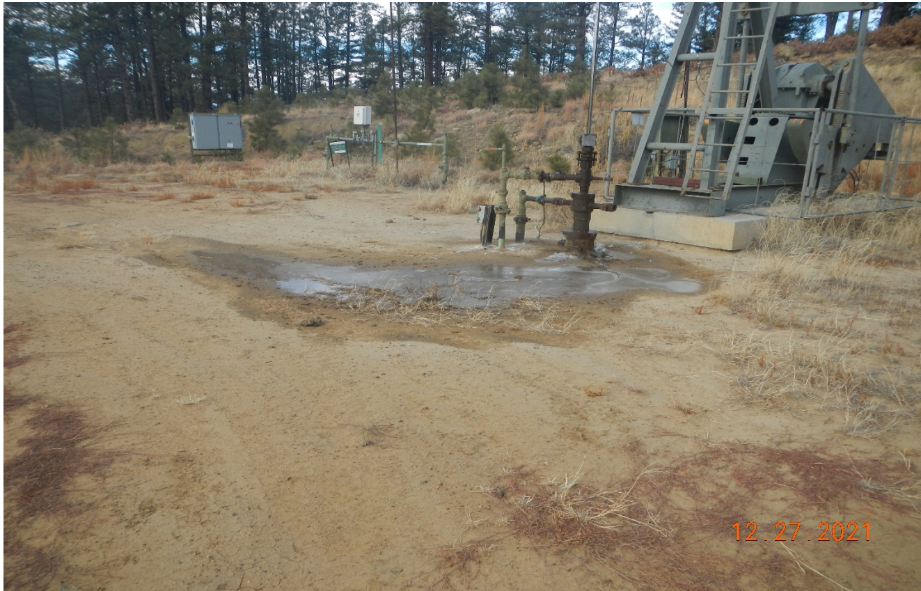
Photo 5. There is a dripping water leak at the wellheads that needs to be fixed.
