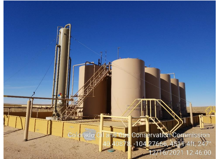
Photo 8 – Tank Battery
