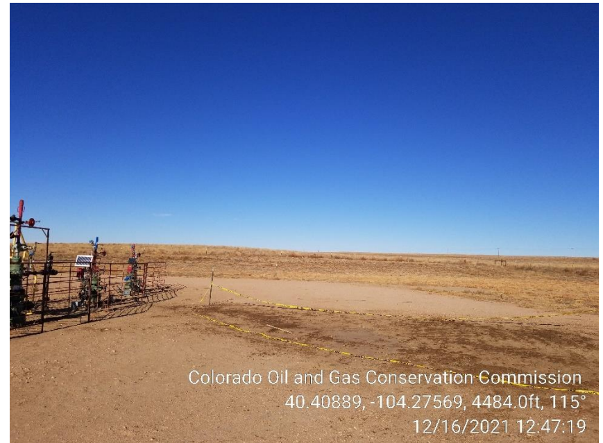
Photo 12 – Stained Soil at Wellheads
