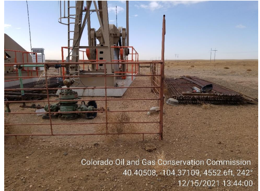
Photo 2 – Wellhead – Unused Rods and Wellhead Parts
