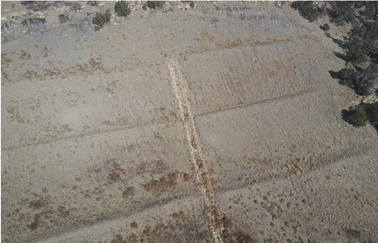
Photo 3. Facing down toward the recontoured location. There are areas of rilling erosion and the berms are not maintained.
