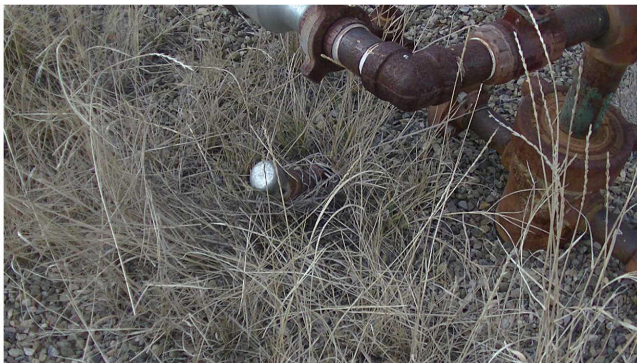
Plumbed Bradenhead to the surface to comply with Rule 608.e.
