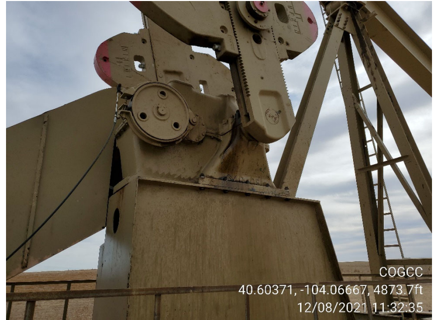
Photo 4 Gearbox leaks
