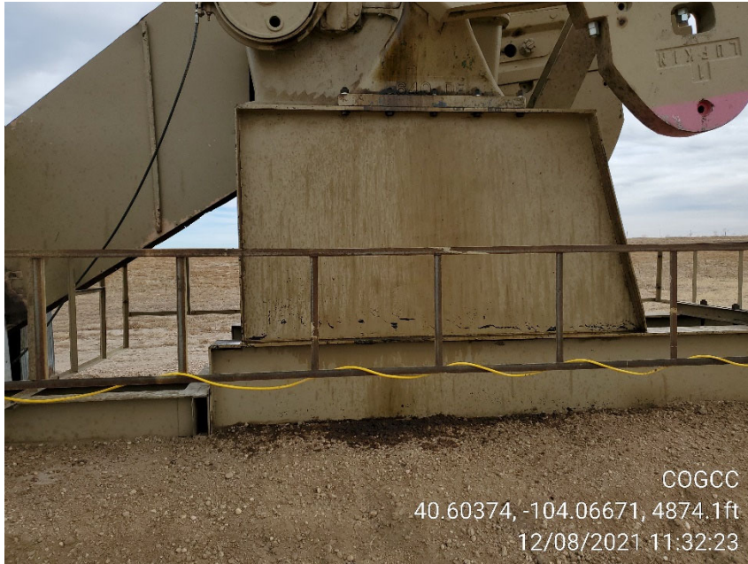
Photo 3 Gearbox leaking onto ground
