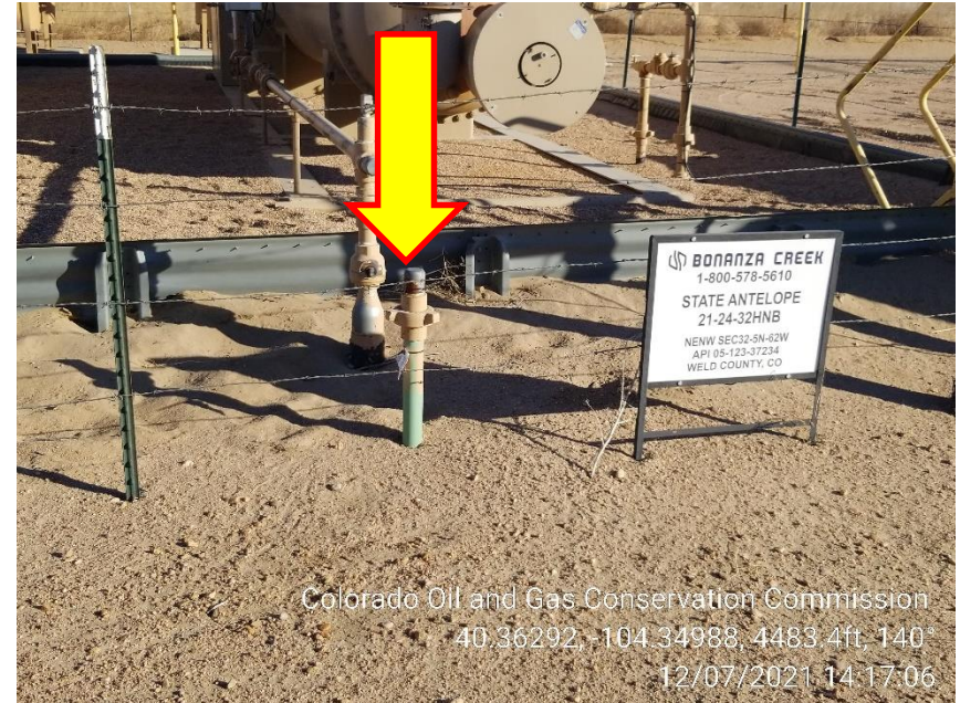
Photo 6 – Unmarked Riser
