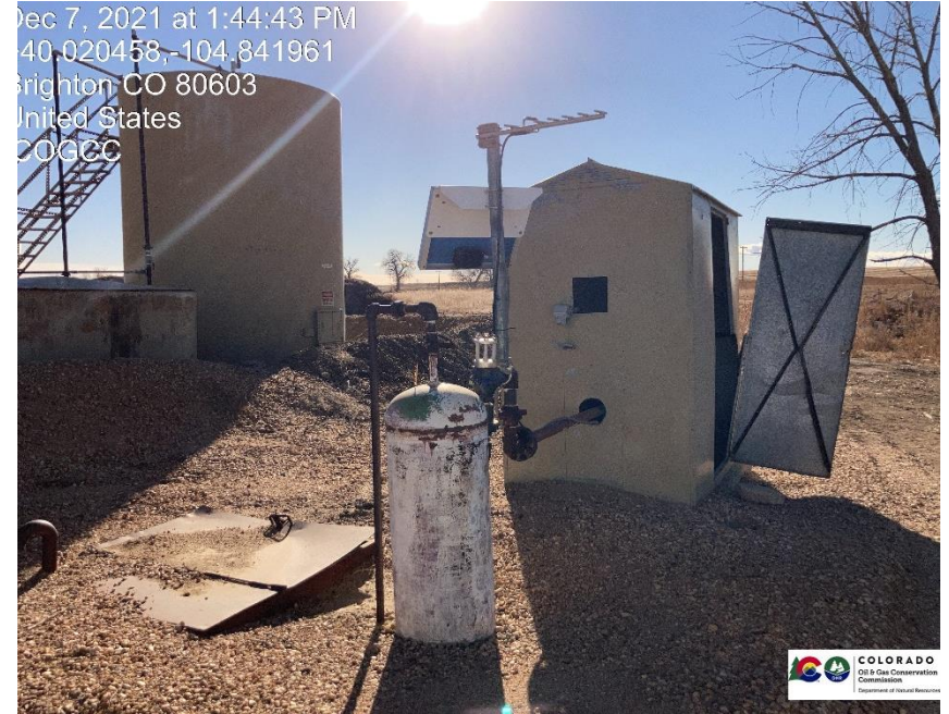
Pic 4 Gas meter run / vertical separator
