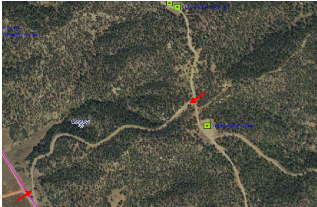
Photo 5. View of the aerial map between the two red arrows is the road shown in photos 1 thru 4. This road is steep and not stabilized as shown in the photos. This section of the road is not necessary for production of the well and needs to be recontoured and reclaimed.
