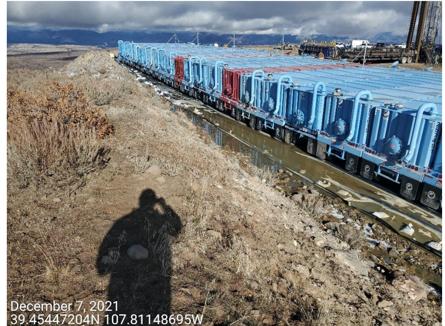
Photo 1: Photo shows containment BMPs at tanks has not been maintained in proper functioning condition.
