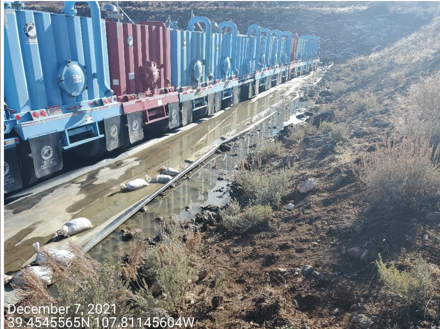
Photo 1: Photo shows containment BMPs at tanks has not been maintained in proper functioning condition.
