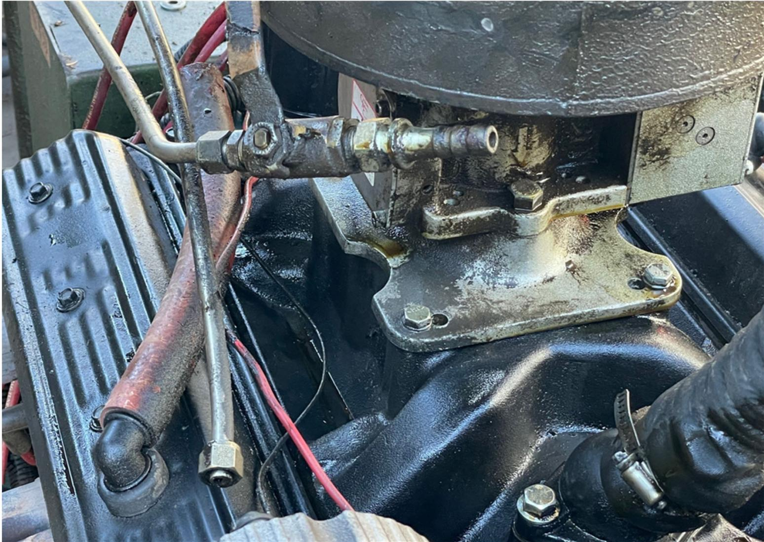
THE LEAK ON THE COMPRESSOR WAS REPAIRED AND THE FLUID ACCUMULATION WAS REMOVED 11/04/2021. A NEW LEAK WAS DETECTED PARTS WERE ORDERED AND REPLCED. UNIT WAS MONTORED FOR A MONTH TO INSURE MAINTENANCE WAS INCLUSIVE.
