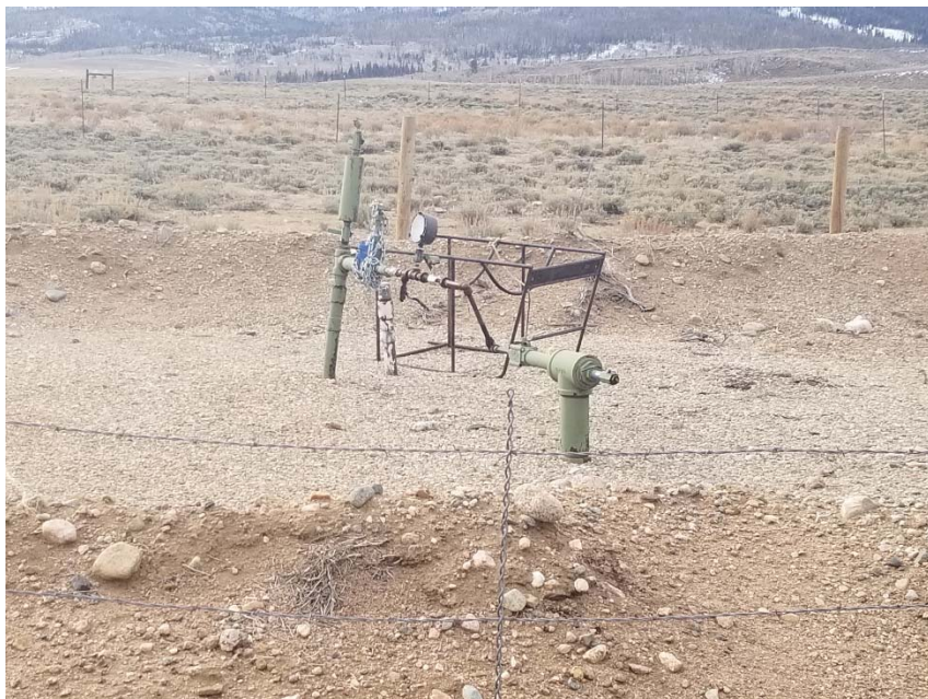
Photo 2. No bradenhead access apparent.
