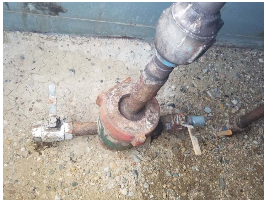
Photo 2. No bradenhead access apparent.
