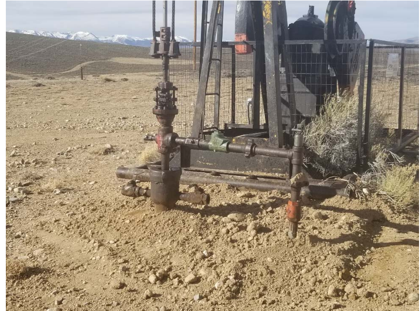
Photo 2. No bradenhead access apparent.
