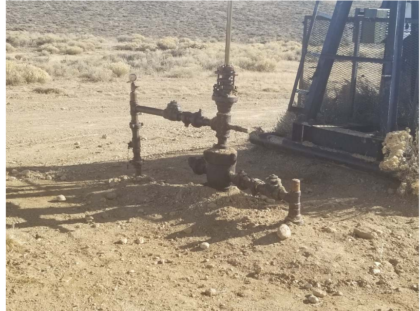
Photo 2. No bradenhead access apparent.
