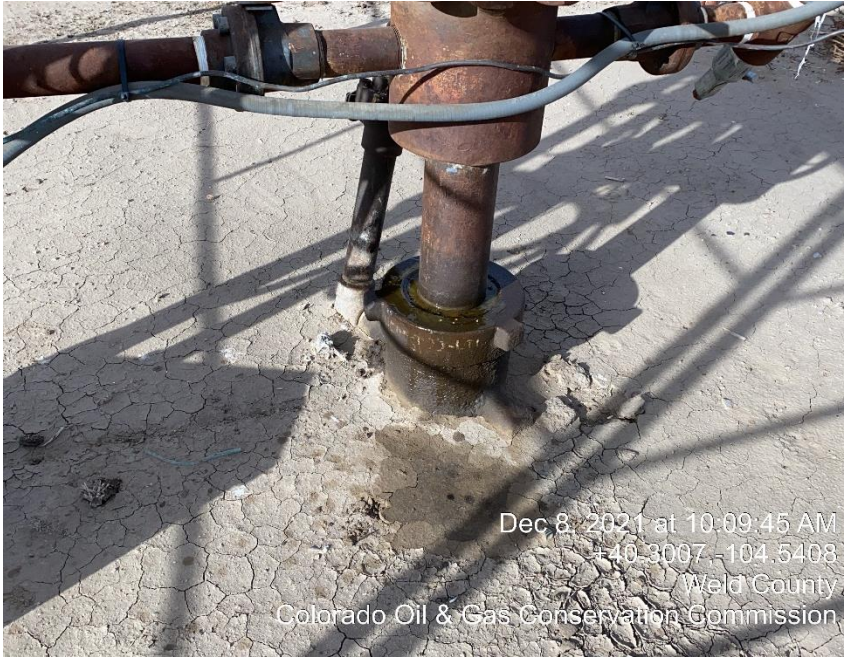
Photo #2 Stained Soil & Appears to be Mechanical Conditions on the Casing Nut.
