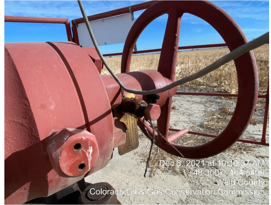
Photo #3 Appears to be Mechanical Conditions on the Packing Screw
