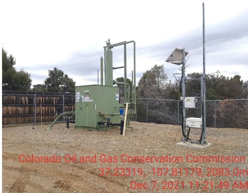
Photo 5 Vert Sep and meter run
