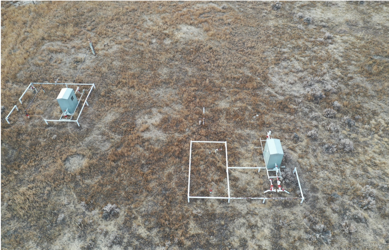
Photo 4. Drone aerial photo down toward the abandoned well site location. There are two abandoned meter runs and equipment that remain at the location.
