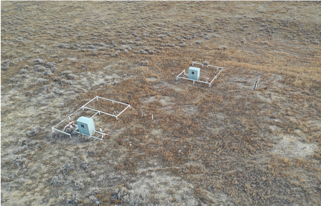
Photo 3. Drone aerial photo down toward the abandoned well site location. There are two abandoned meter runs and equipment that remain at the location.
