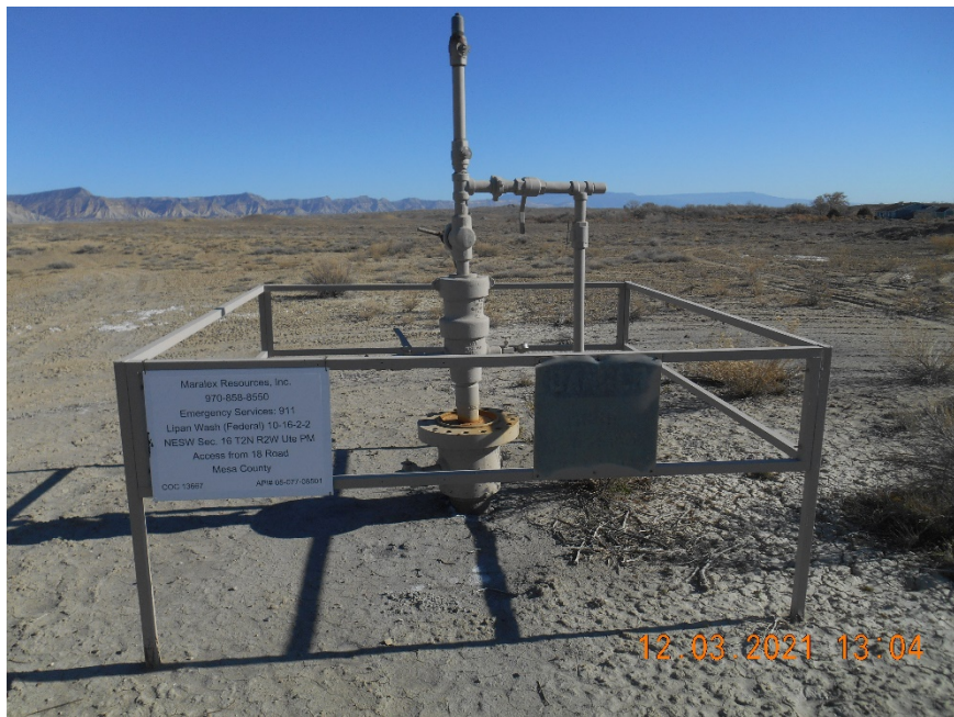
Wellhead with fencing and sign
