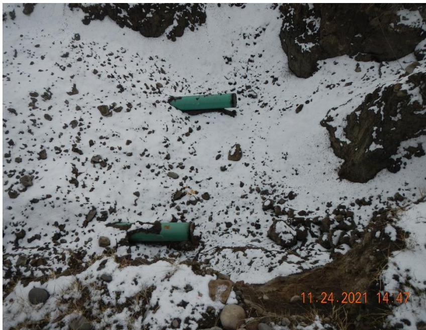
Flow lines with welded on caps near location entrance.
