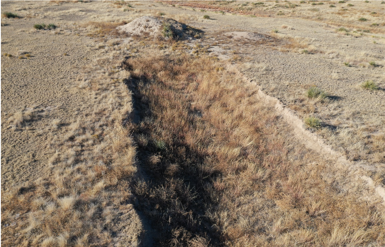
Photo 4. Facing northwest toward a lined pit which is approximately 100'x30' in size. There is degraded liner debris that remains in the pit.
