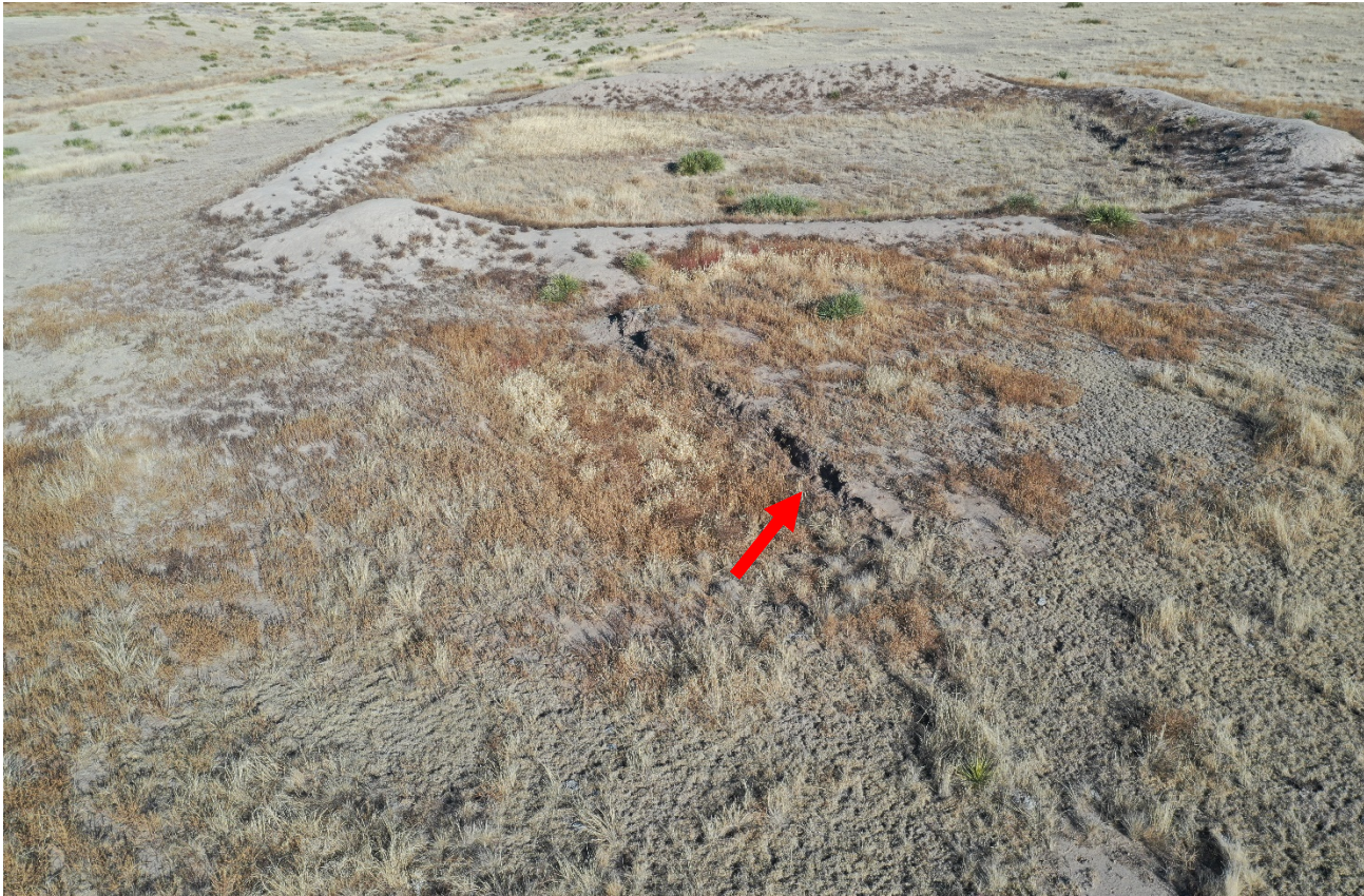
Photo 3. Facing northeast toward the pit. There is trench shown at red arrow which is diverted toward the pit from the location of the abandoned well. This area was never backfilled and reclaimed.
