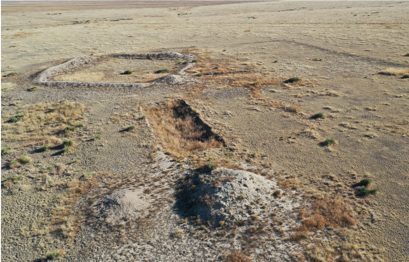
Photo 5. Drone aerial photo facing southeast toward the abandoned well location. The pits were never backfilled and reclaimed.
