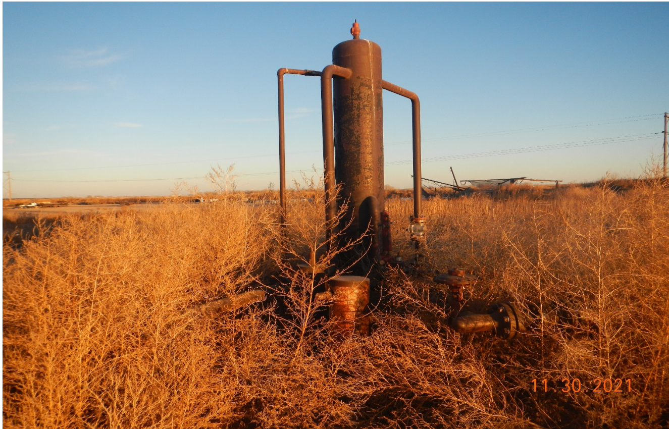
Photo 1. Facing east. There is abandoned gas separator that remains at the location. There is also undesirable weeds growing around the abandoned equipment.
