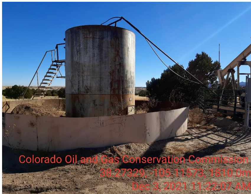
Photo 3 no markings, placards on crude oil tank
