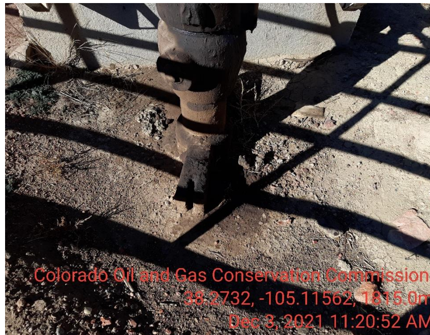
Photo 2 stained soil around well head
